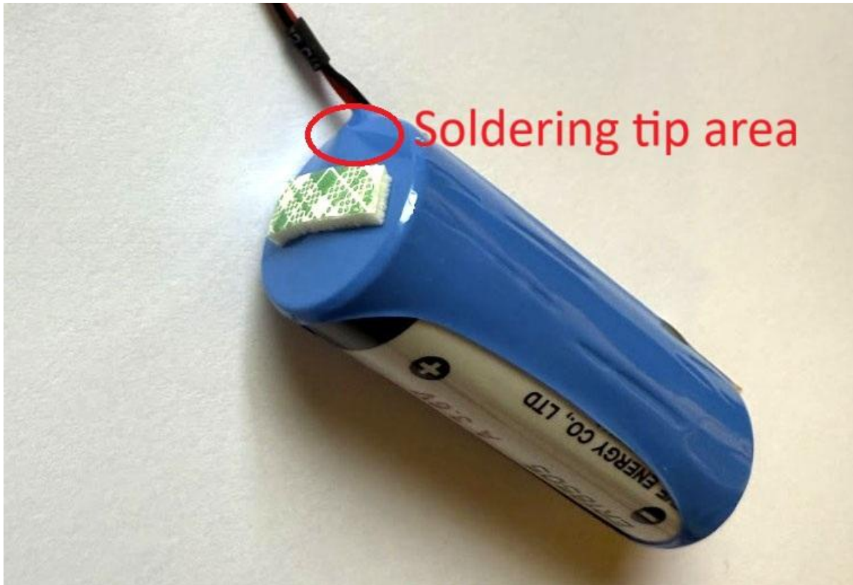
Figure 11 Add double-sided foam to battery positive terminal. Avoid covering the soldering tip area
