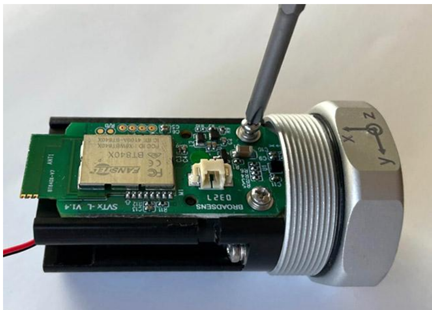
Figure 7 Remove two screws on PCBA
