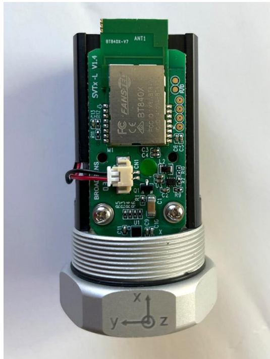
Figure 5 Internal SVT-L/SAG sensor
