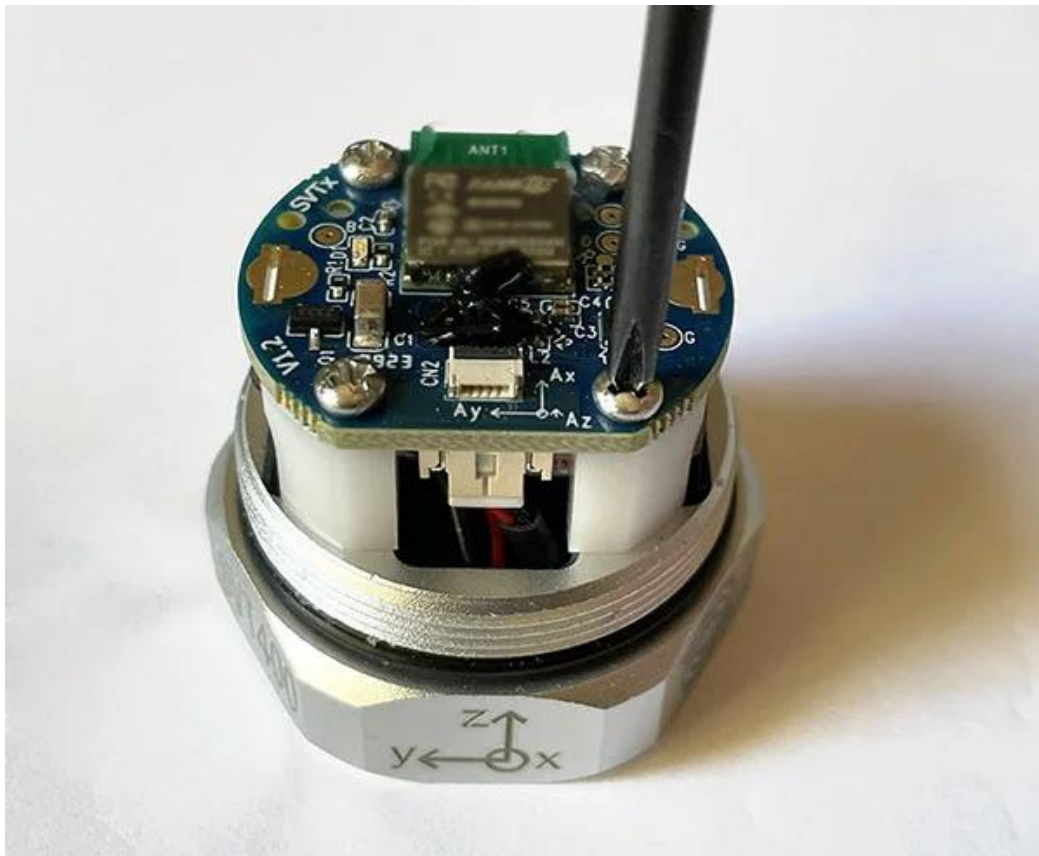
Figure 1 Remove four screws that fix the PCBA to the battery cover
