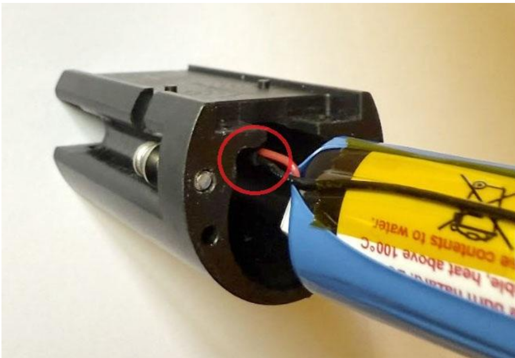
Figure 13 Insert the battery and let the battery wires go inside the groove
