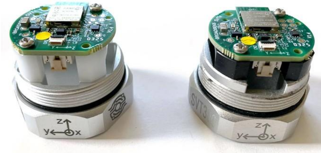
Figure 2 Sensor internal (left: old design; right: new design)
