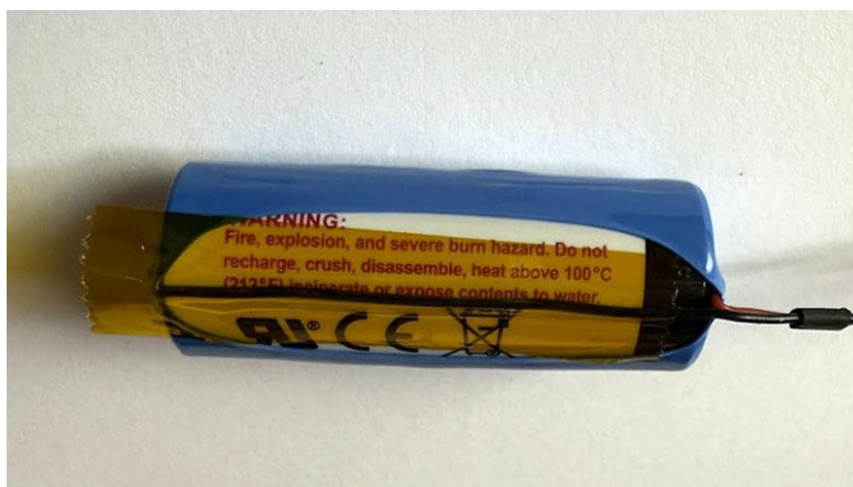
Figure 10 Fix battery wire with heat resistant tape
