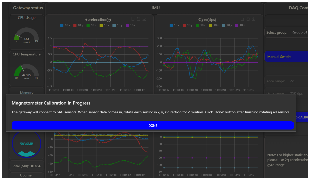
Figure 106 Magnetometer calibration in progress
