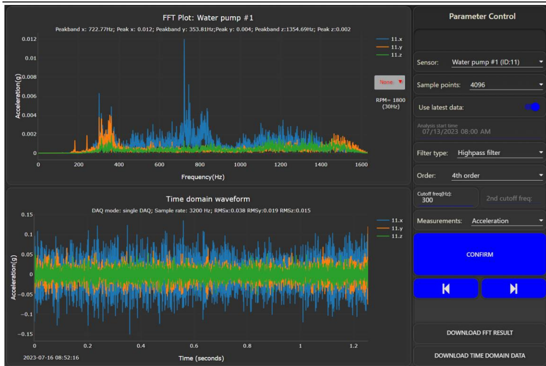
Figure 60 4 th order High pass filter applied to signal
