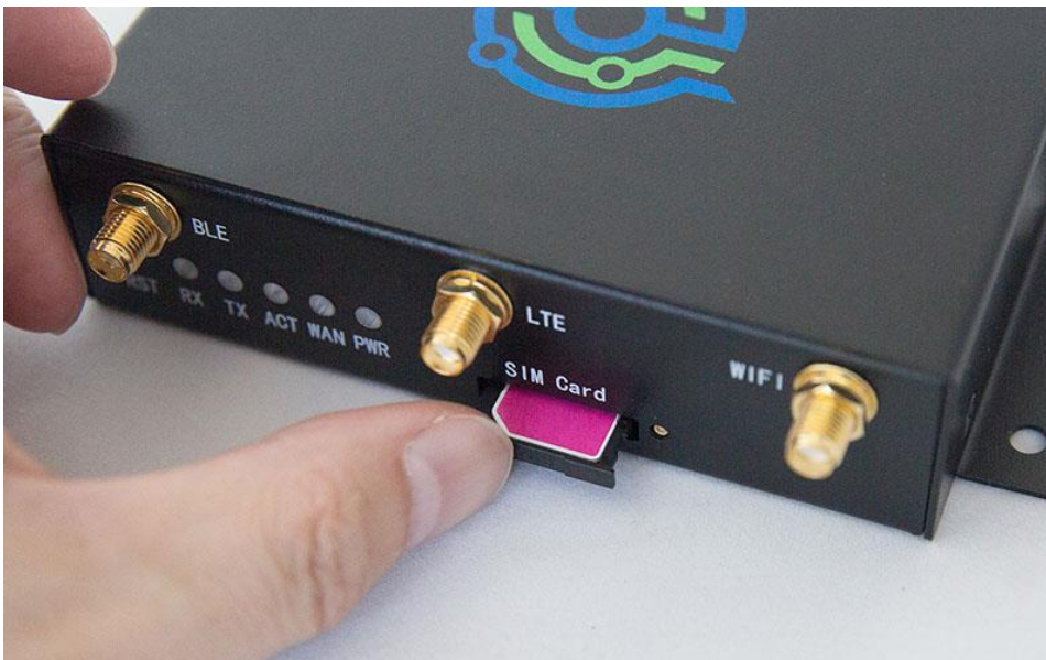
Figure 11 Insert SIM card tray to GU300S
