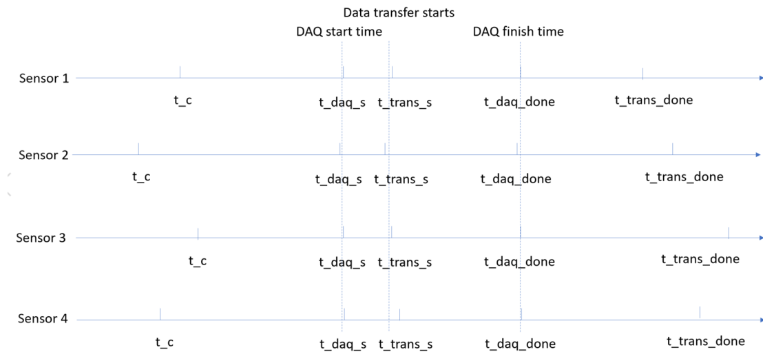
Figure 31 Synchronized single DAQ mode timing
