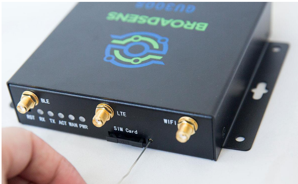
Figure 9 Eject SIM card tray from GU300S
